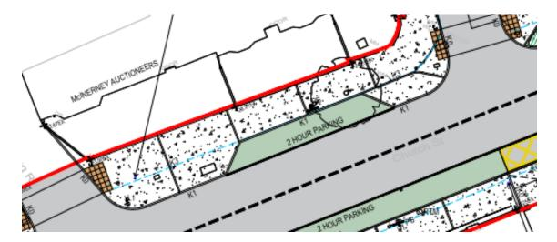
**Hazard:** Riders of powered two-wheeled vehicles may lose vehicle control when attempting to cross the kerb. Additionally high sided vehicles in the parking bay may restrict visibility on exit from the driveways.
