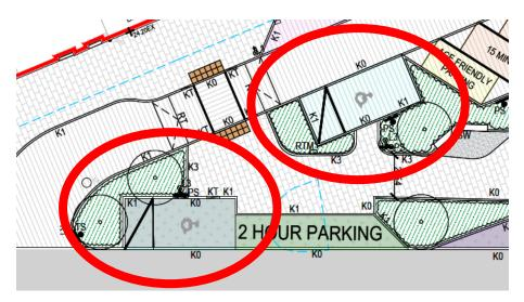
**Hazard:** Disabled users without direct access to the footpath may be required to travel on the carriageway prior to accessing the footpath. Impact from passing vehicles may result.
